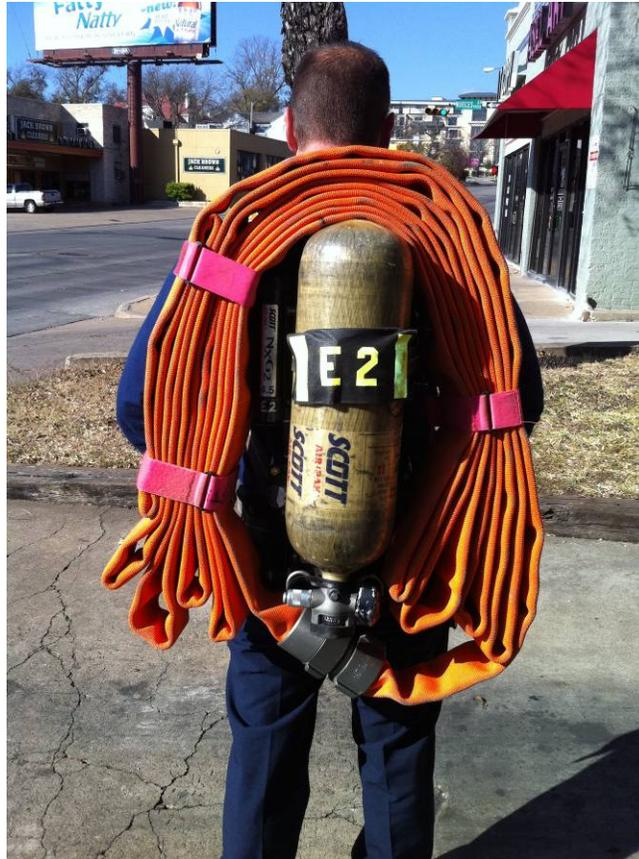
*The hose fold over the air pack serves two purposes. First, it distributes the weight much more efficiently, thus making it easier on the firefighter. Secondly, both hands are now free to carry other tools and equipment. By starting the hose fold at 32"- 36", the completed fold fits nicely over the air pack.*
