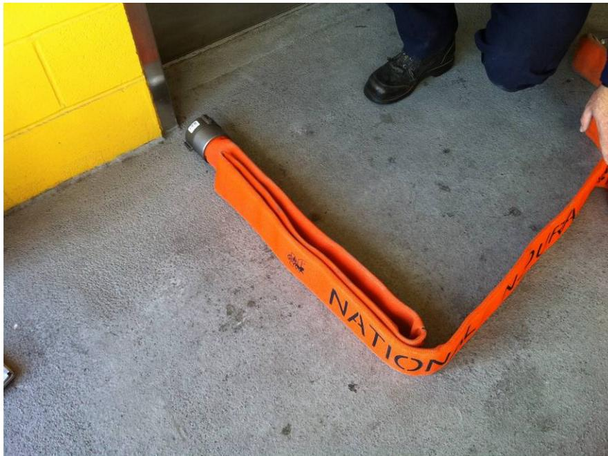
*The fold is taken 32”- 36” from the end of the female coupling. This may seem too short, but as the fold is completed a proper length will be maintained.*
